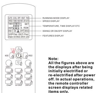
The **cooling only units** don't have the function of heating or electric heating. When the remote controller turns to such function buttons, the units will not result such effect. \*Please don't turn the remote controller to such buttons.
